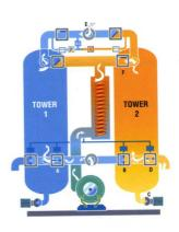
Towers filled with extra, high-grade activated alumina to deliver superior performance
